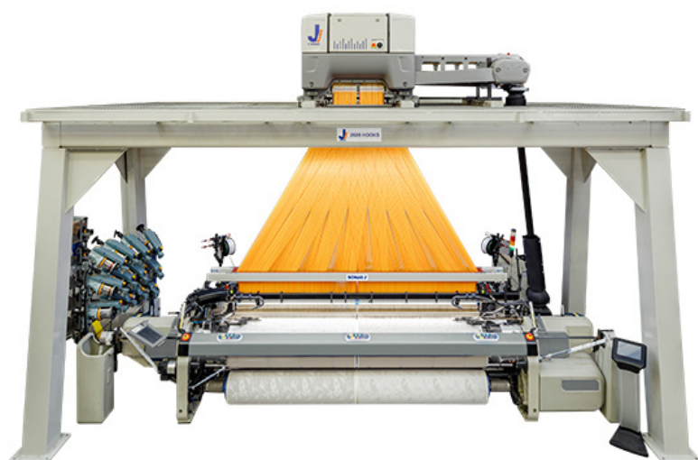
Figure 3: Ji jacquard with 2.688 hooks on top of a rapier loom weaving designs on double width in 8 repeats
