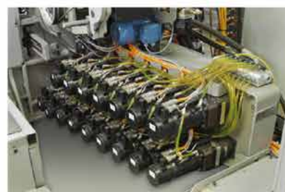
SF Smart Frames: electronic shedding by servomotor
