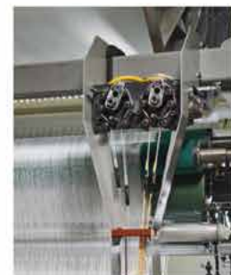
SE Smart Edges for servomotor selvedge control
