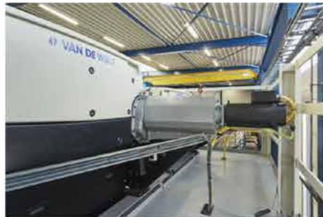
Servodrive Jacquard with electronic timing adjustment
